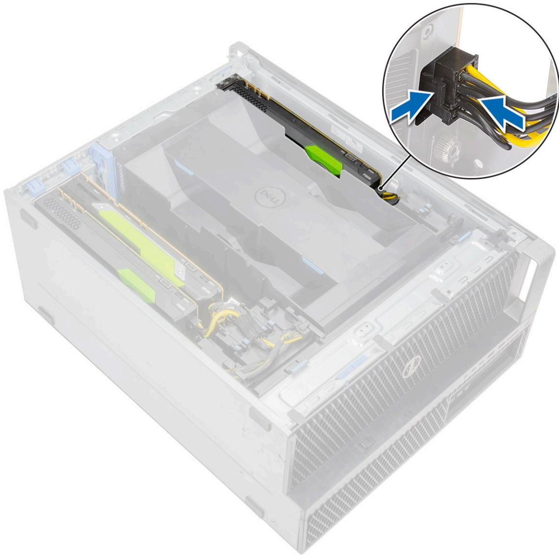
g Press and rotate the PCIe latch backward to unlock the filler bracket.
