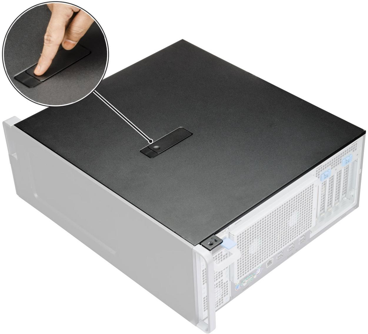
b Pull the latch [1] upward and slide the side cover outwards to remove it from the system [2].
